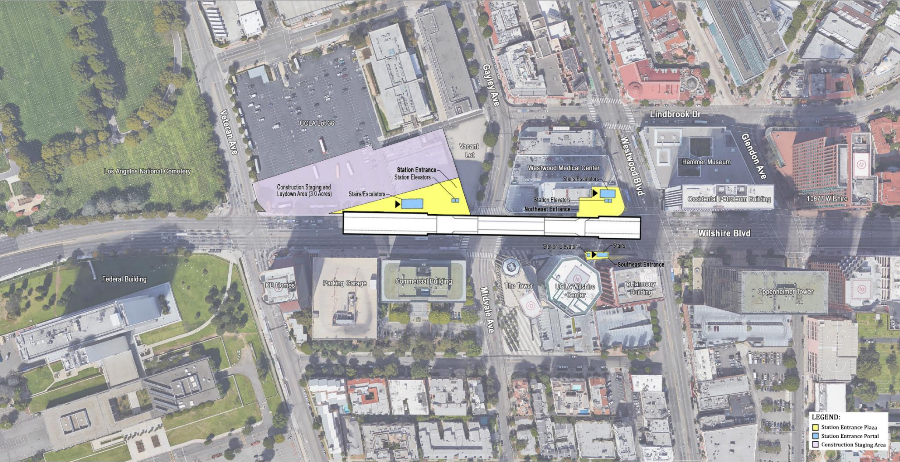
The underground station box under Wilshire Bl between Westwood Bl and Veteran Av. is approximately 902 feet long, and 64 feet wide.
