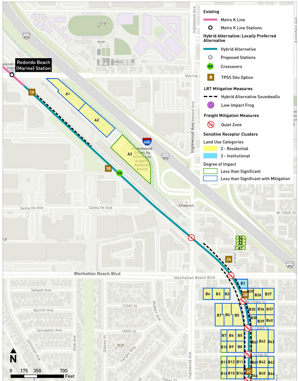
Figure 4-5. LPA - Mitigated Operational Noise Impacts (1 of 5)
