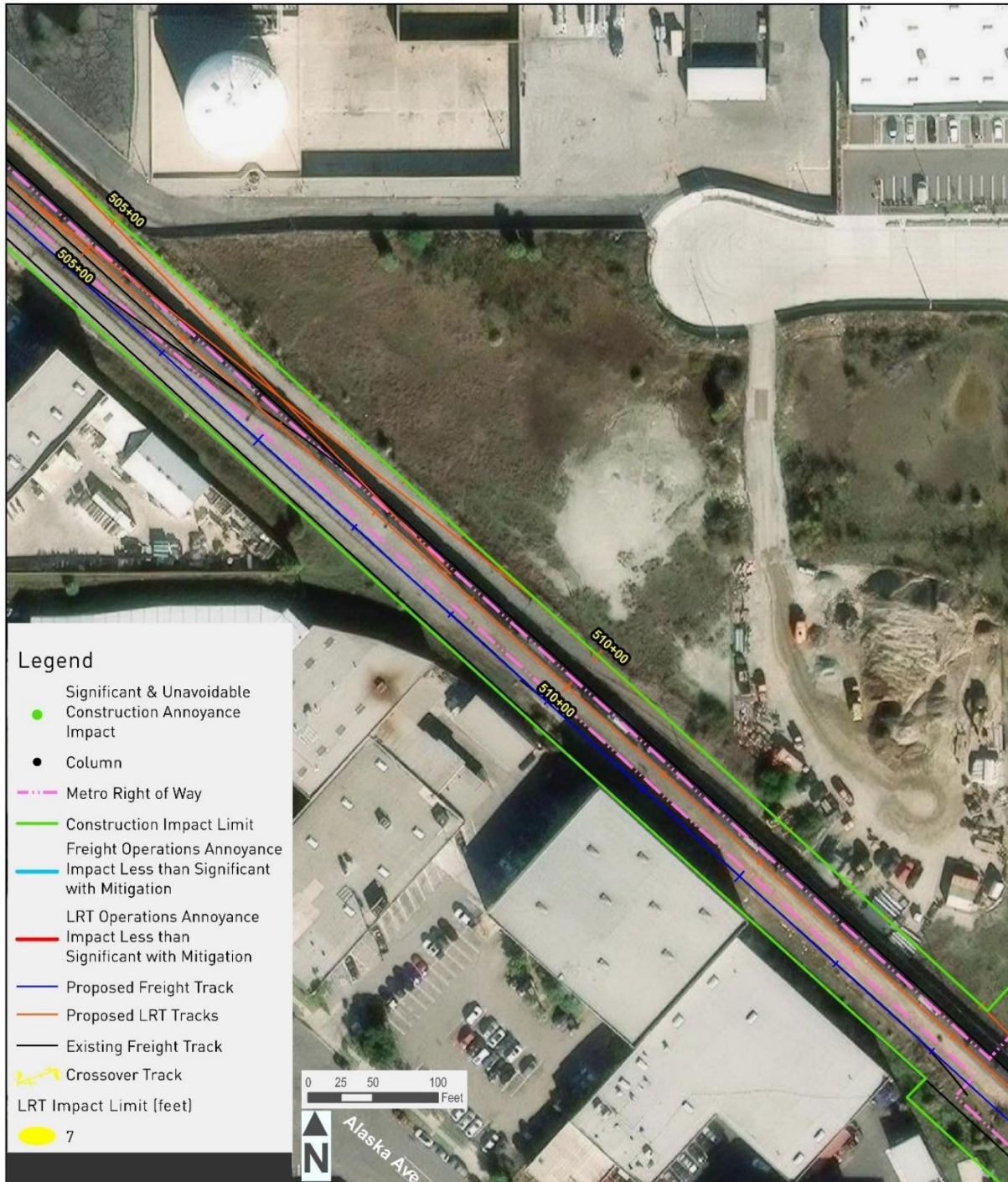
Figure 4-41. LPA Construction & Operation Vibration Impacts 32 of 33
