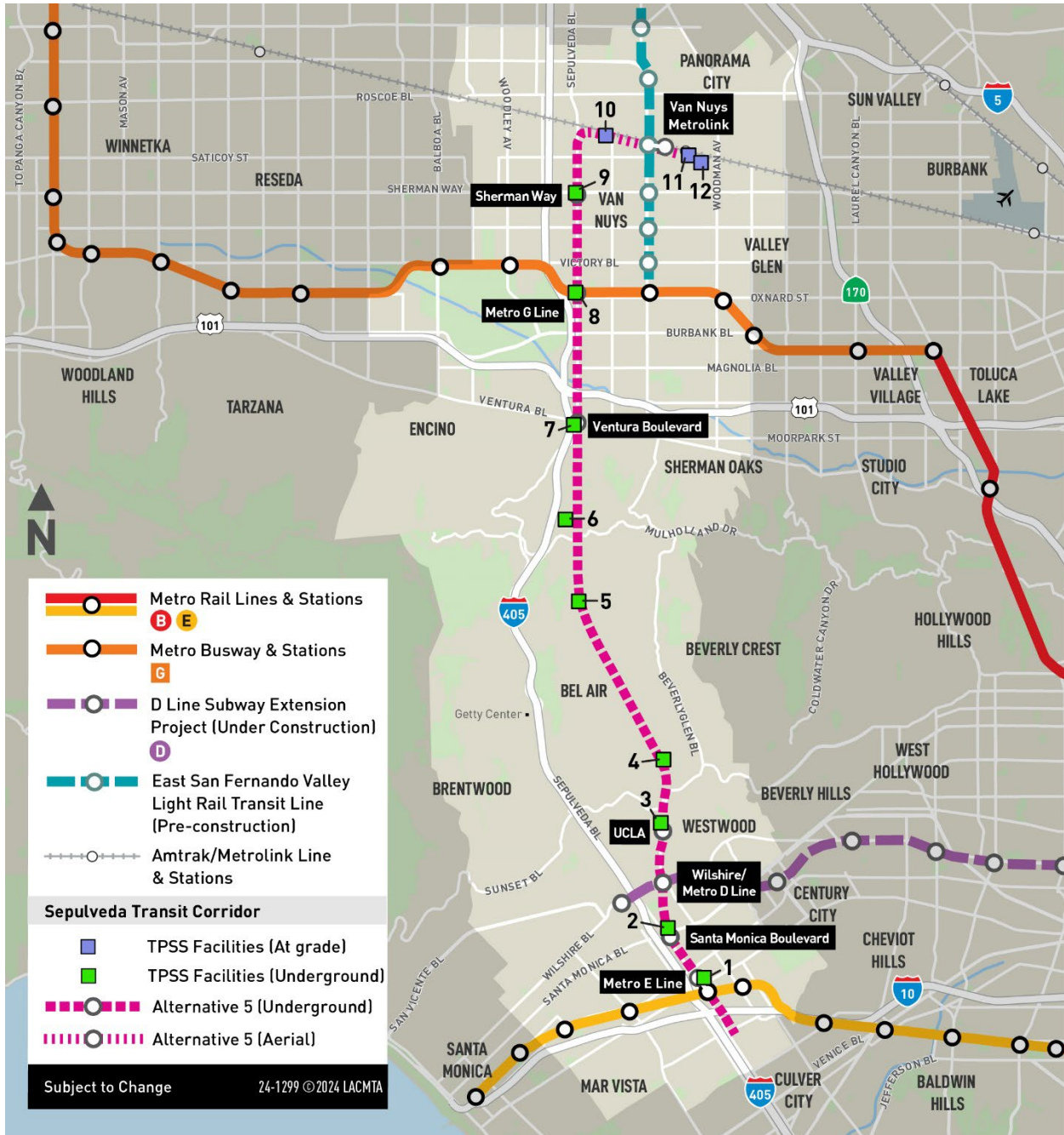
Figure 9-5. Alternative 5: Traction Power Substation Locations
