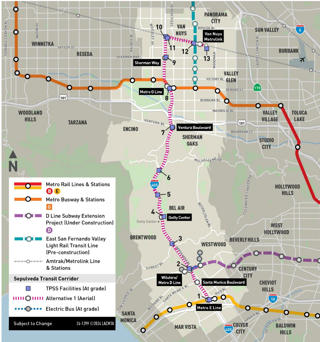
Figure 6-7. Alternative 1: Traction Power Substation Locations
