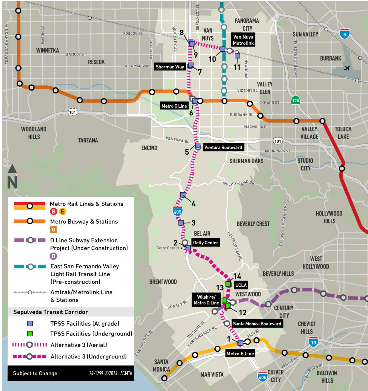
Figure 7-7. Alternative 3: Traction Power Substation Locations
