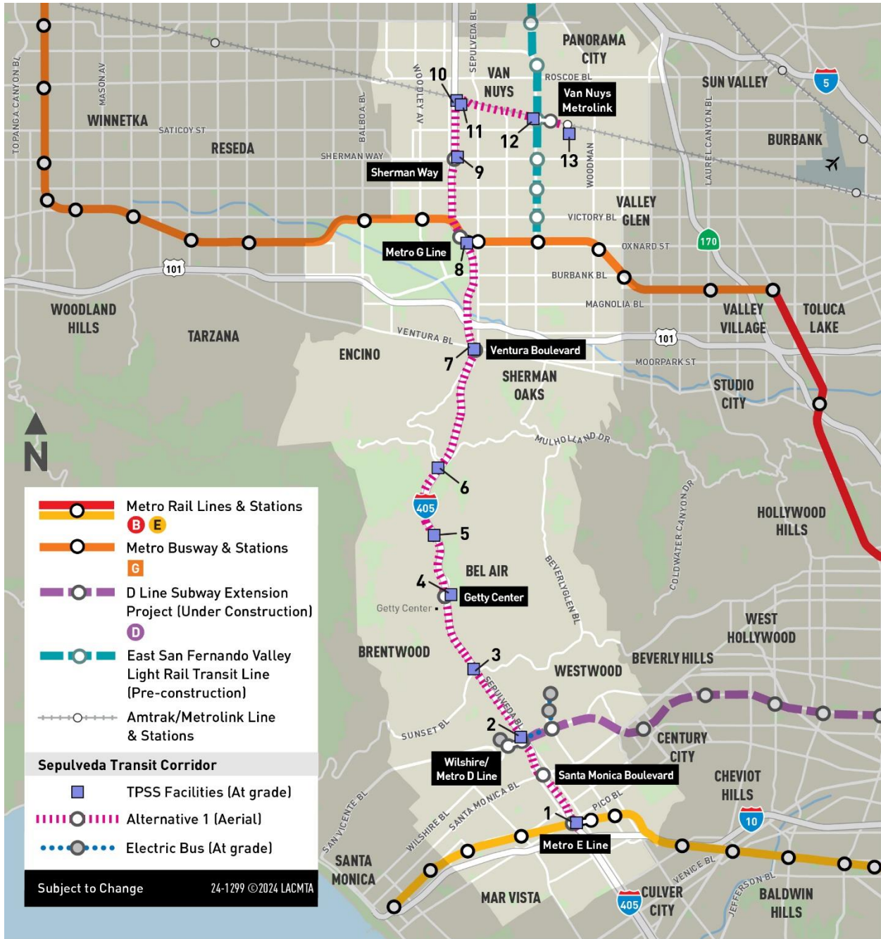
Figure 6-7. Alternative 1: Traction Power Substation Locations
