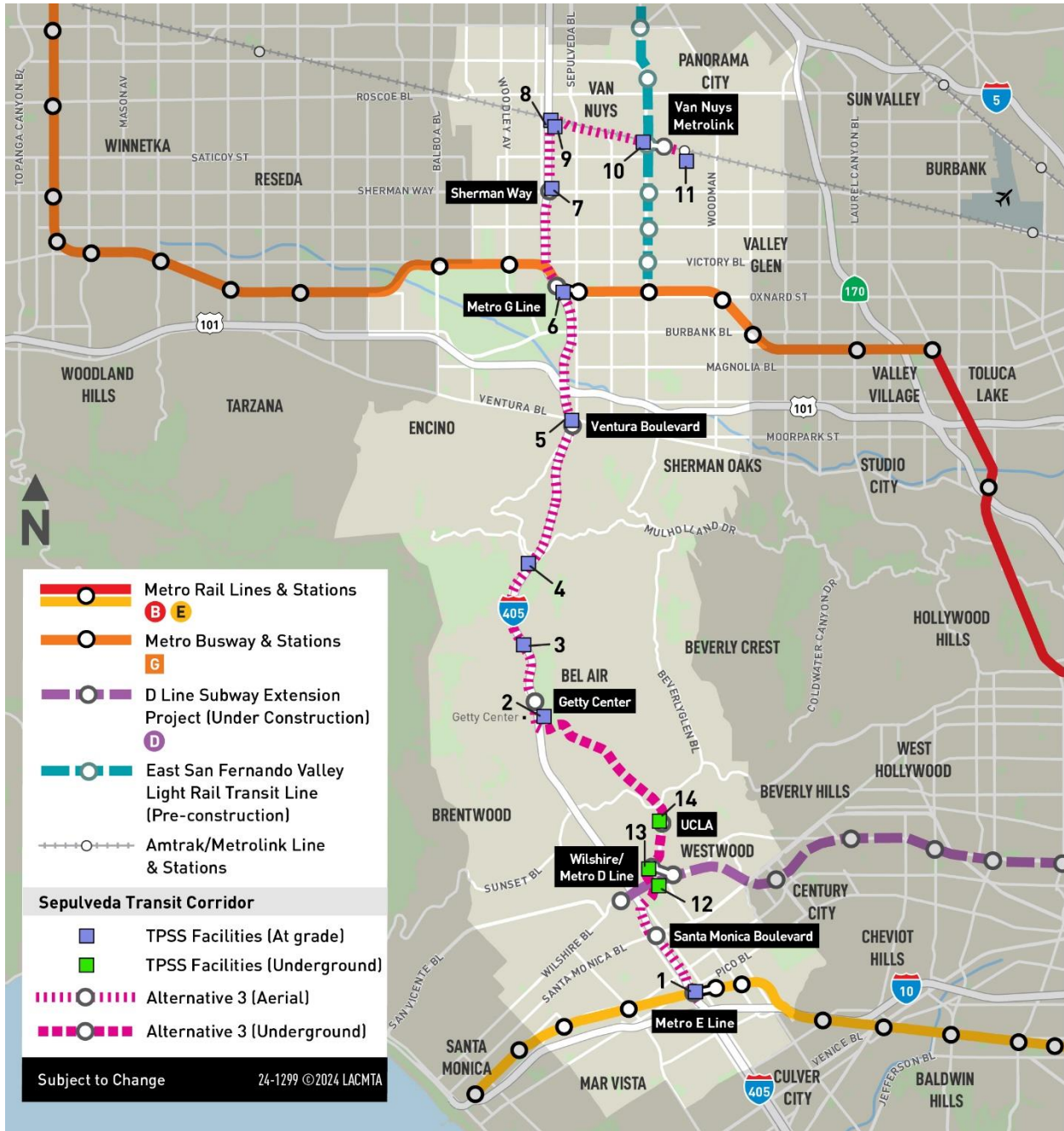
Figure 7-7. Alternative 3: Traction Power Substation Locations
