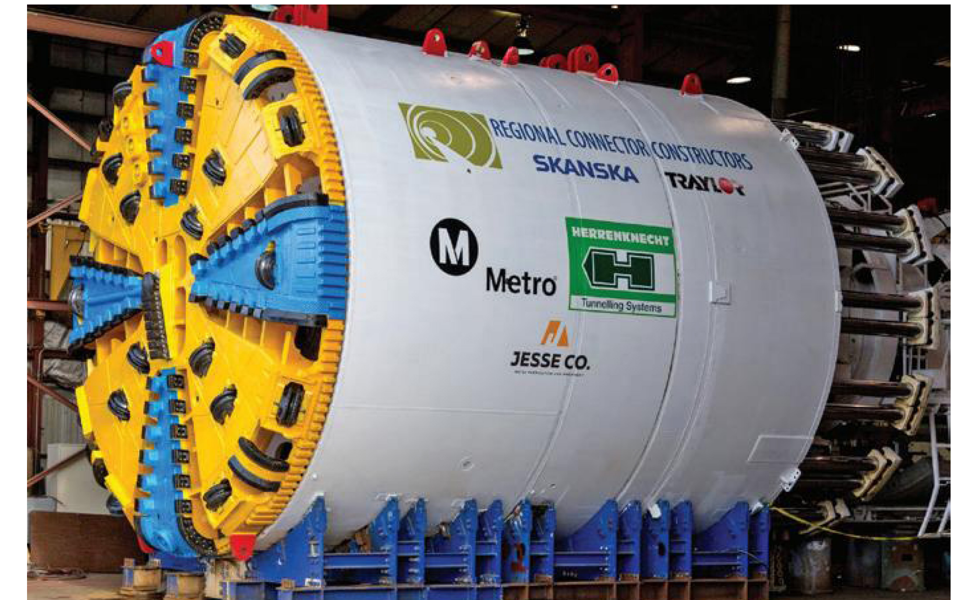
Metro's TBM used on the Regional Connector.
