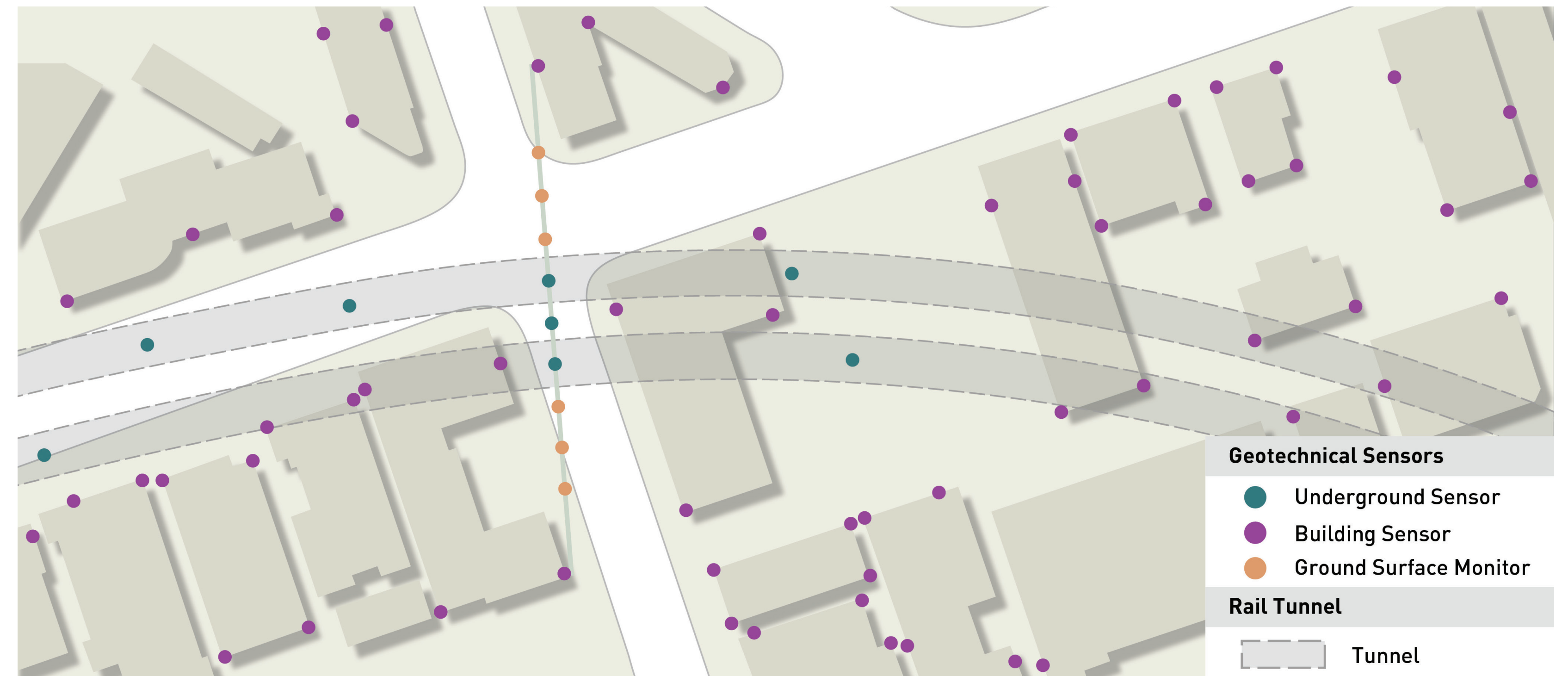
Typical sensor placement.
