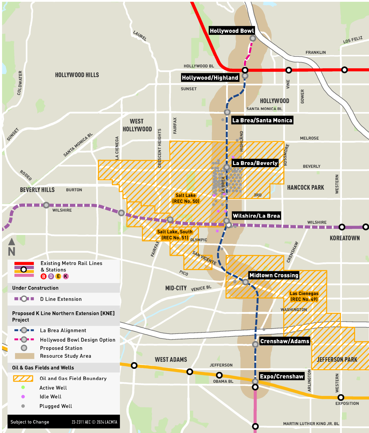
FIGURE 3.11-25. OIL AND GAS FIELDS IN VICINITY OF KNE LA BREA ALIGNMENT
