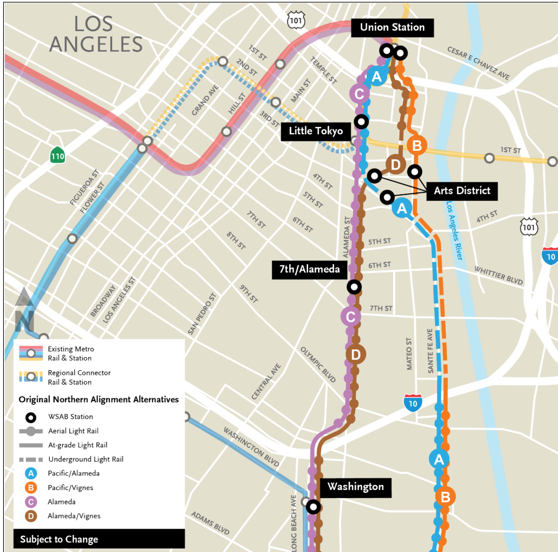
Figure 4-1. WSAB Transit Corridor Original Northern Alignment Alternatives
