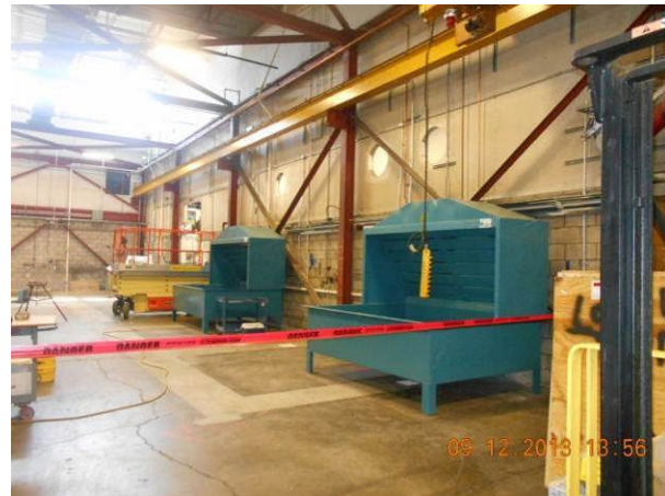
Radiator leak test tanks at New Radiator Shop.
