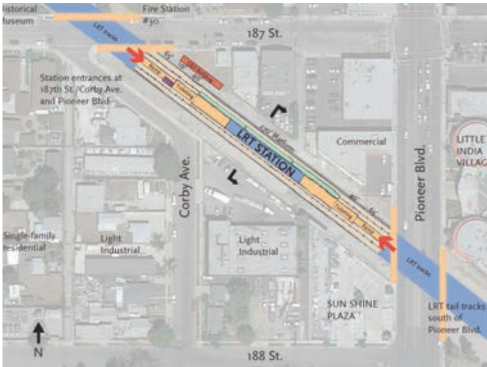
Figure 2-35: The preferred plan accommodates the Southern Terminus station platform between 187th Street and Pioneer Boulevard
