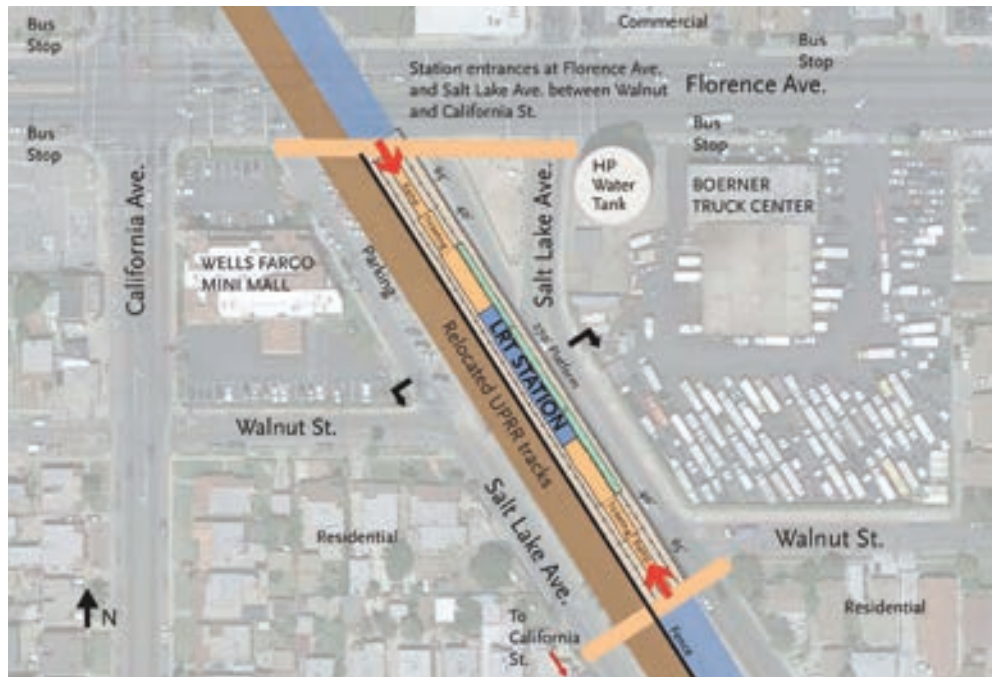
Figure 2-18: Conceptual plan for a center platform station at Florence Avenue in Huntington Park
