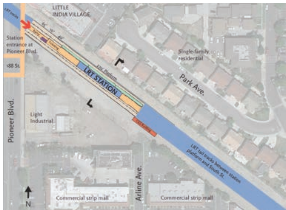
Figure 2-34: One of two options developed accommodates the Southern Terminus station platform east of Pioneer Boulevard but was not preferred by the Cities of Artesia or Cerritos
