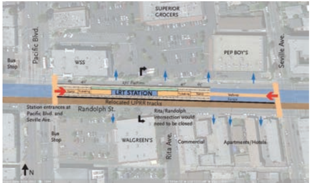
Figure 2-14: Conceptual plan for a center platform station on Randolph Street in Huntington Park
