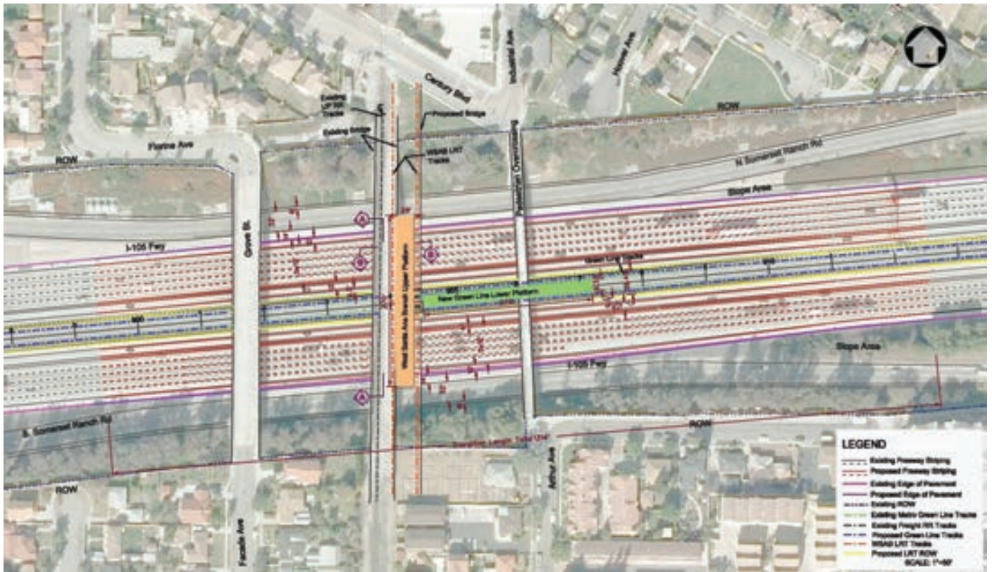
Figure 2-29: Potential freeway lane configuration (non-standard) for new Metro Green Line Station and WSAB/Green Line Station
