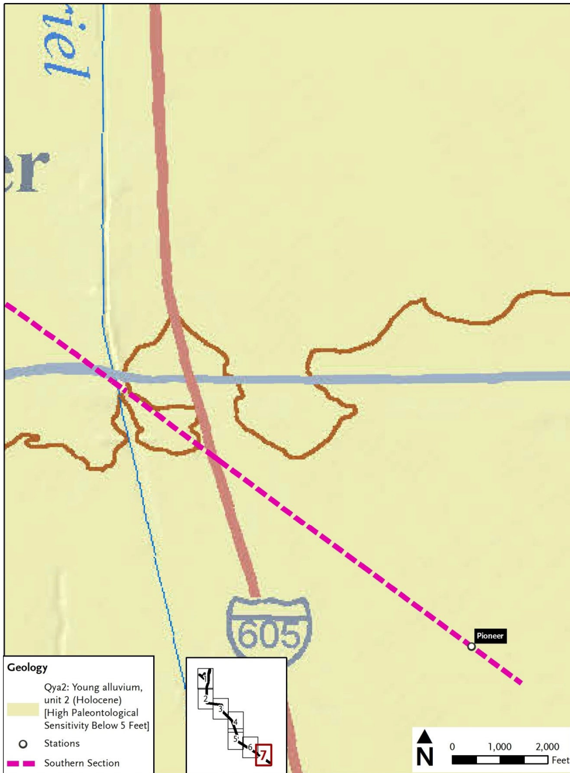
Figure B-8. Geologic Units and Paleontological Sensitivity in the Affected Area, Sheet 7
