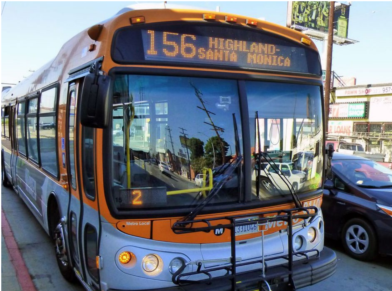
Typical Metro head sign with route number, route name and destination displayed. Color and contrast increase legibility from a distance. Photo Credit: Jonathan Riley
