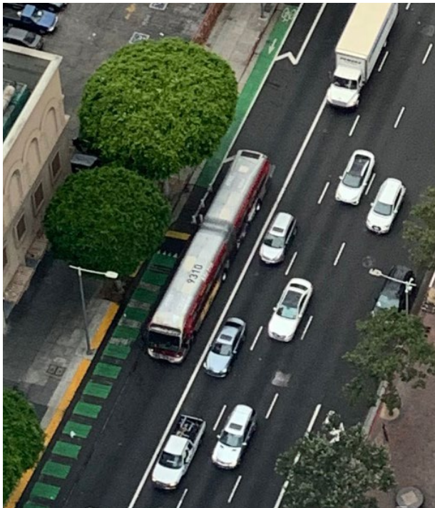
Paint used to delineate shared station use between bikes and bus - Los Angeles, CA - Photo Credit: IBI Group
