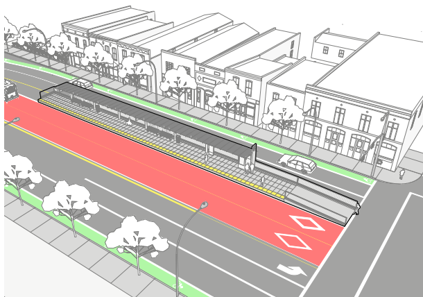
Center Running – Side/Side Staggered Station
