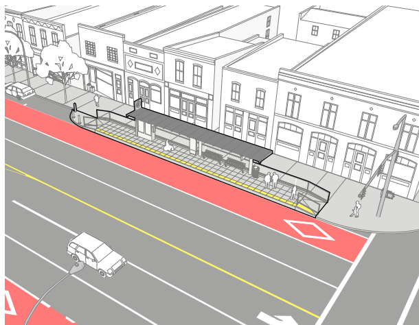
Side Running – Bulbout Attached Station
