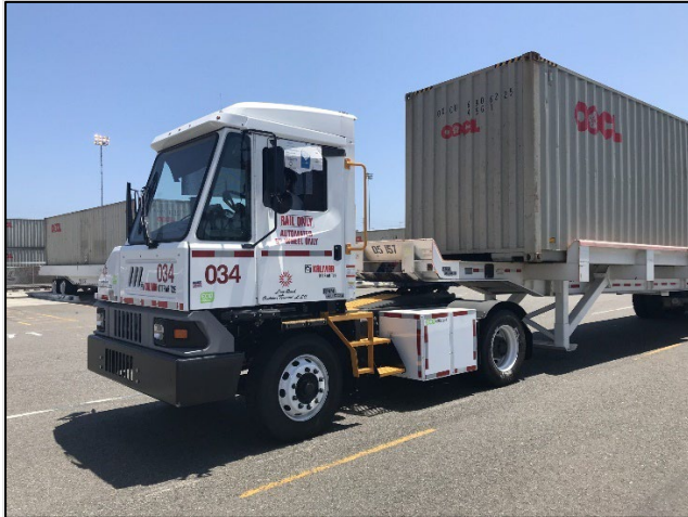
Utility Tractor Rig (UTR). Semi-tractor used to move trailers within a cargo yard, warehouse facility, or intermodal facility.
