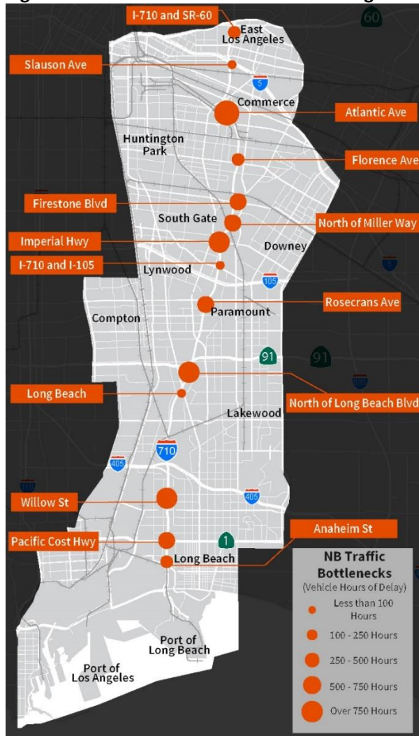
Figure 3-68. Northbound Bottlenecks Along I-710
