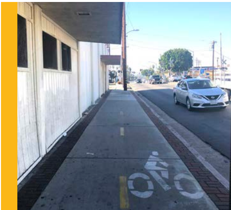
Bike path incorporated into the sidewalk
