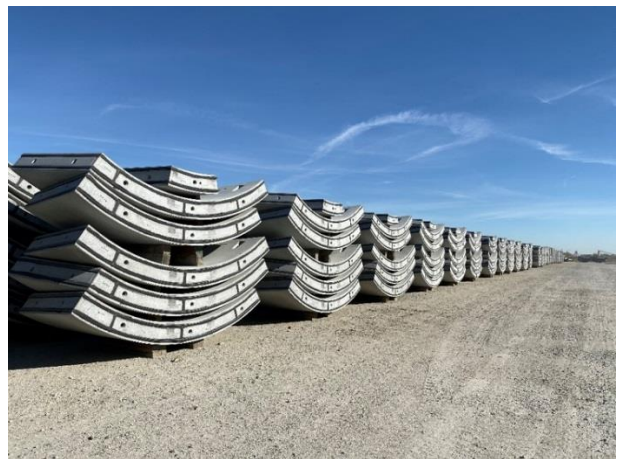
Precast Tunnel Access Rings in Little Rock, CA
