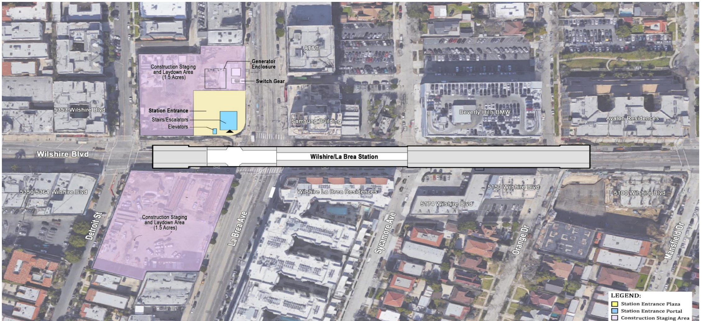
Outline of the Wilshire/La Brea underground station box on Wilshire Bl. from Orange Dr. to Detroit St.
