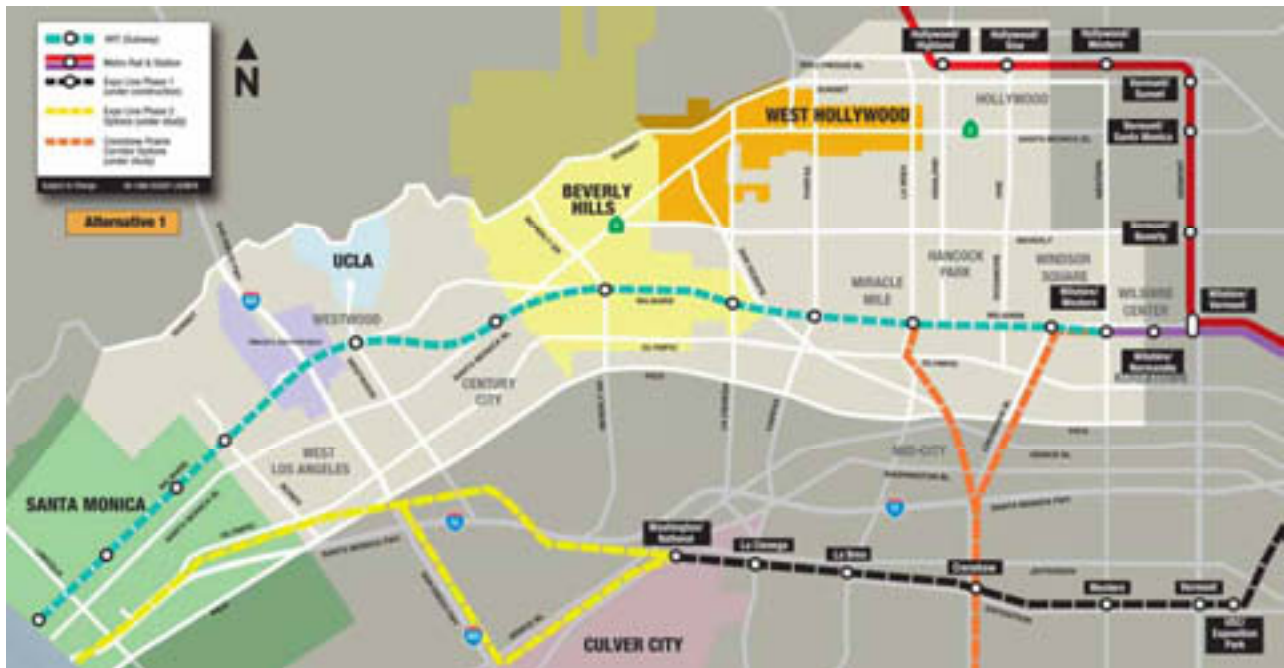
Figure 2-10. Alternative 1 – Wilshire Boulevard Alignment HRT Subway
