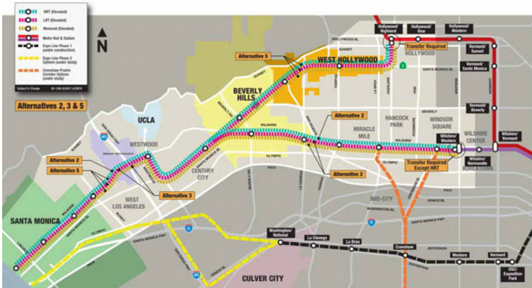
Figure 2-27. HRT, LRT and Monorail Elevated Alternatives
