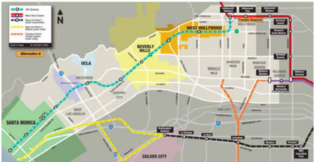
Figure 2-15. Alternative 6 – Santa Monica Boulevard Alignment HRT Subway with Hollywood/Highland Red Line Connection
