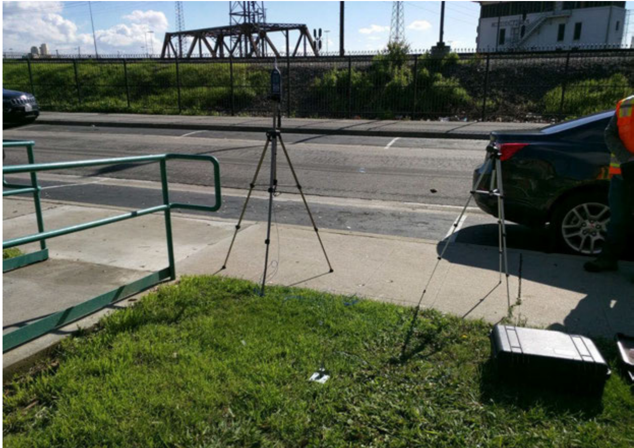
Figure 7-11. Monitoring Location 1a – Vibration Measurement at William Mead Homes
