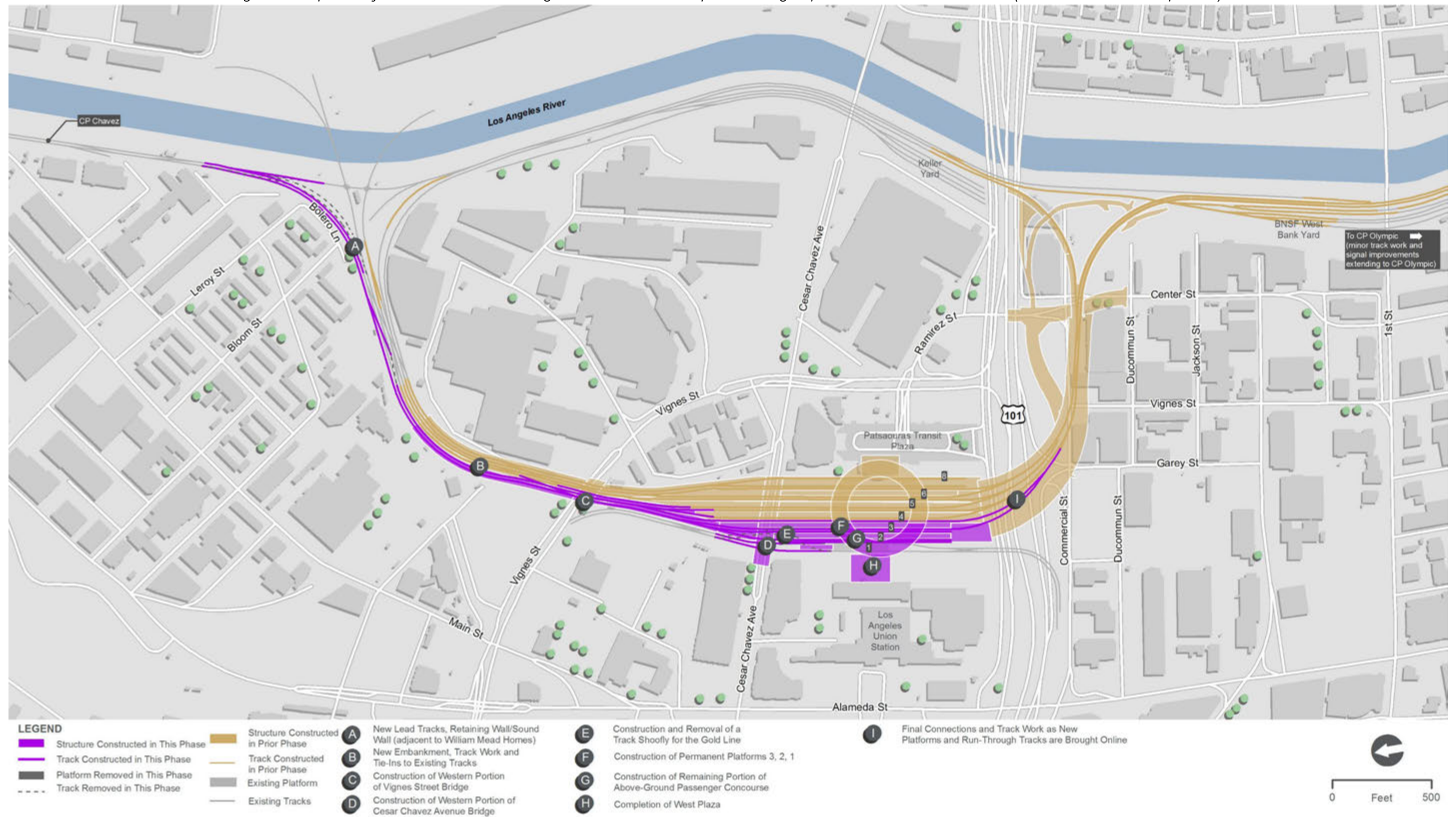
Figure 7-9. Proposed Project with Above-Grade Passenger Concourse with New Expanded Passageway – Detailed Construction Scenario (Phase IV Construction Steps 18-22)
