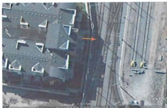
Fusion Figure 1-4: Photo, from Google Earth, of distance of planned and future tracks to Division 22 site, from Northeastern-most building in Fusion complex. Distance from Patio to middle of MTA track is 22 feet.
