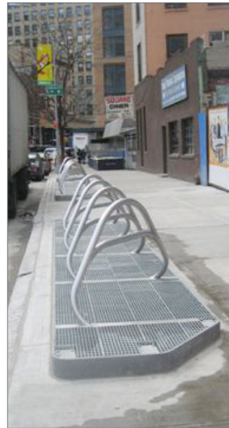
◀ (Left) Air conditioning and heating shafts should be on the roof of transit stations or hidden from view; (Right) Bike racks can be stationed on top of exposed ventilation grates on the ground.
