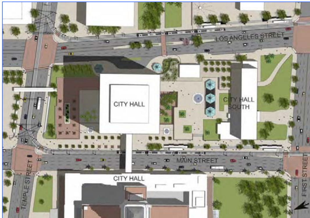
Figure 2-26 At-Grade Emphasis LRT Options A & B – Split station at City Hall along Los Angeles and Main Streets
