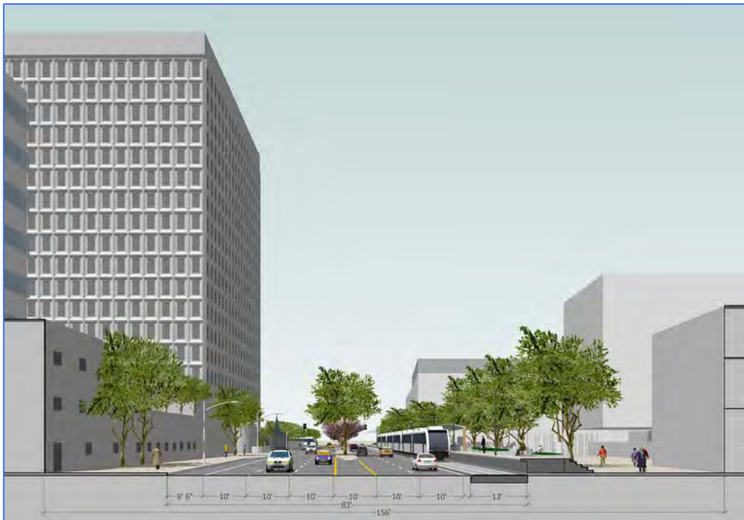
Figure 2-30 At-Grade Emphasis LRT Options A & B – Los Angeles St. looking north from 1 st St.
