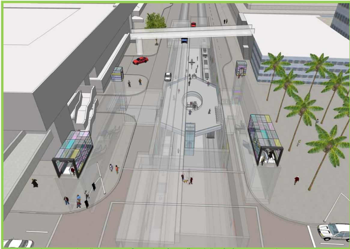
Underground-running tracks will eliminate conflicts with surface traffic and allow for faster train speeds.
