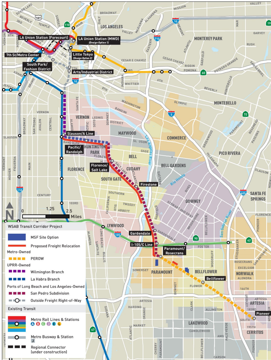
Figure 2-6. Existing Rail Right-of-Way Ownership and Relocation
