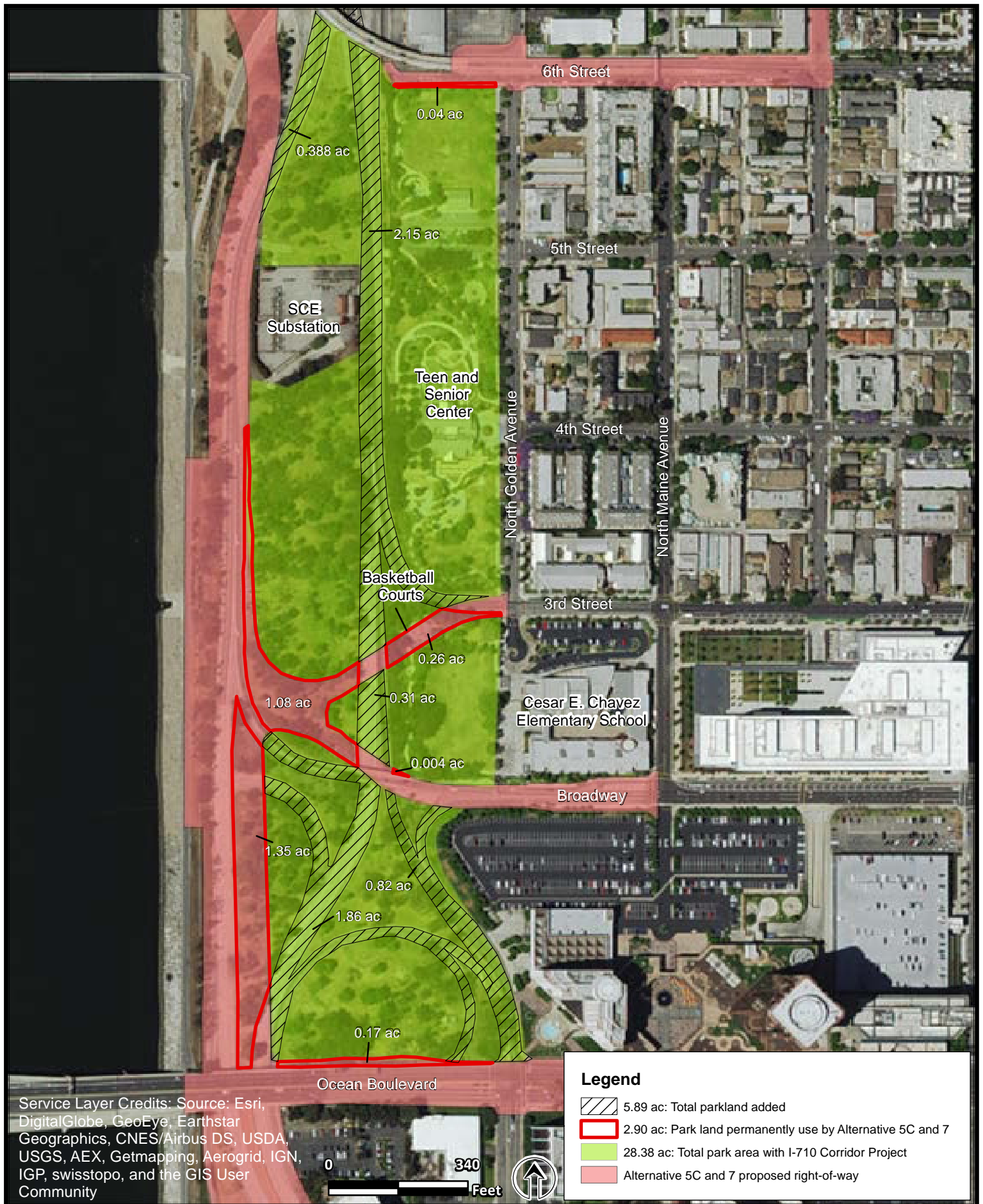
FIGURE 5-1. PERMANENT USE OF LAND AT CESAR E. CHAVEZ PARK ALTERNATIVE 5C AND ALTERNATIVE 7 I-710 Corridor
