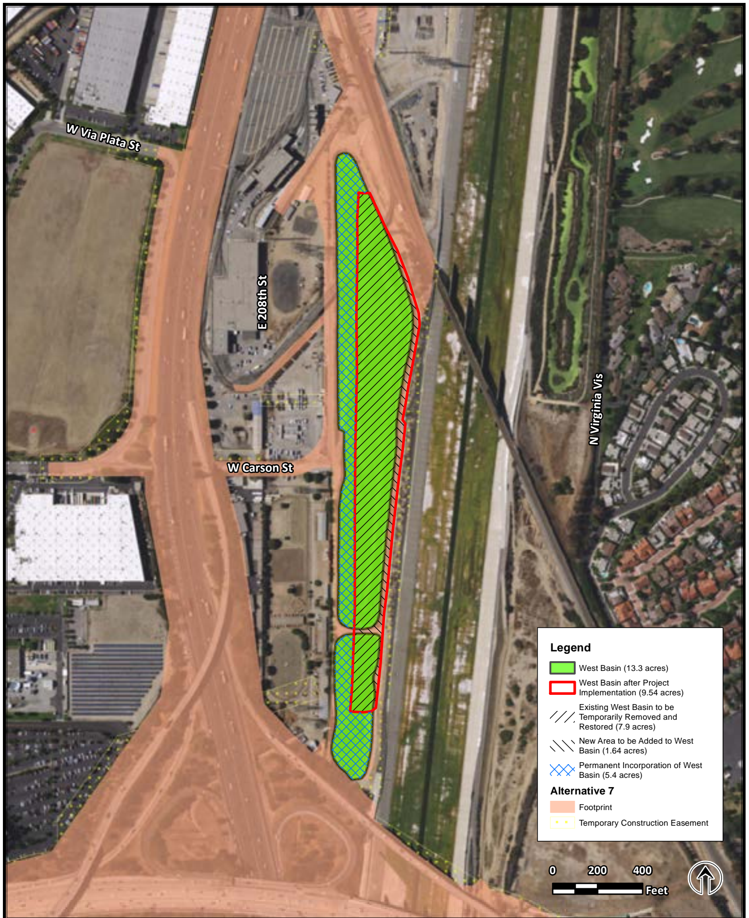
FIGURE 5-2. Impacts on the Dominguez Gap Wetlands, West Basin (ALTERNATIVE 7) I-710 Corridor Project
