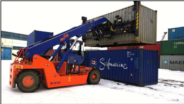
Side Pick. A flexible front or side loader that can reach up to multiple stacks of containers.
