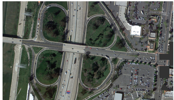
The “cloverleaf” interchanges built in the 1950’s are not able to handle today’s volume of traffic.
