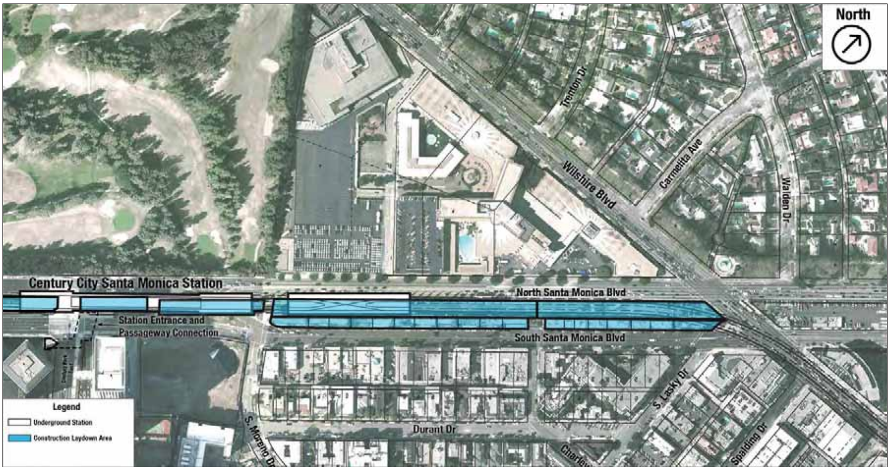
Century City Santa Monica Station – Construction Staging and Laydown Areas Scenario B
