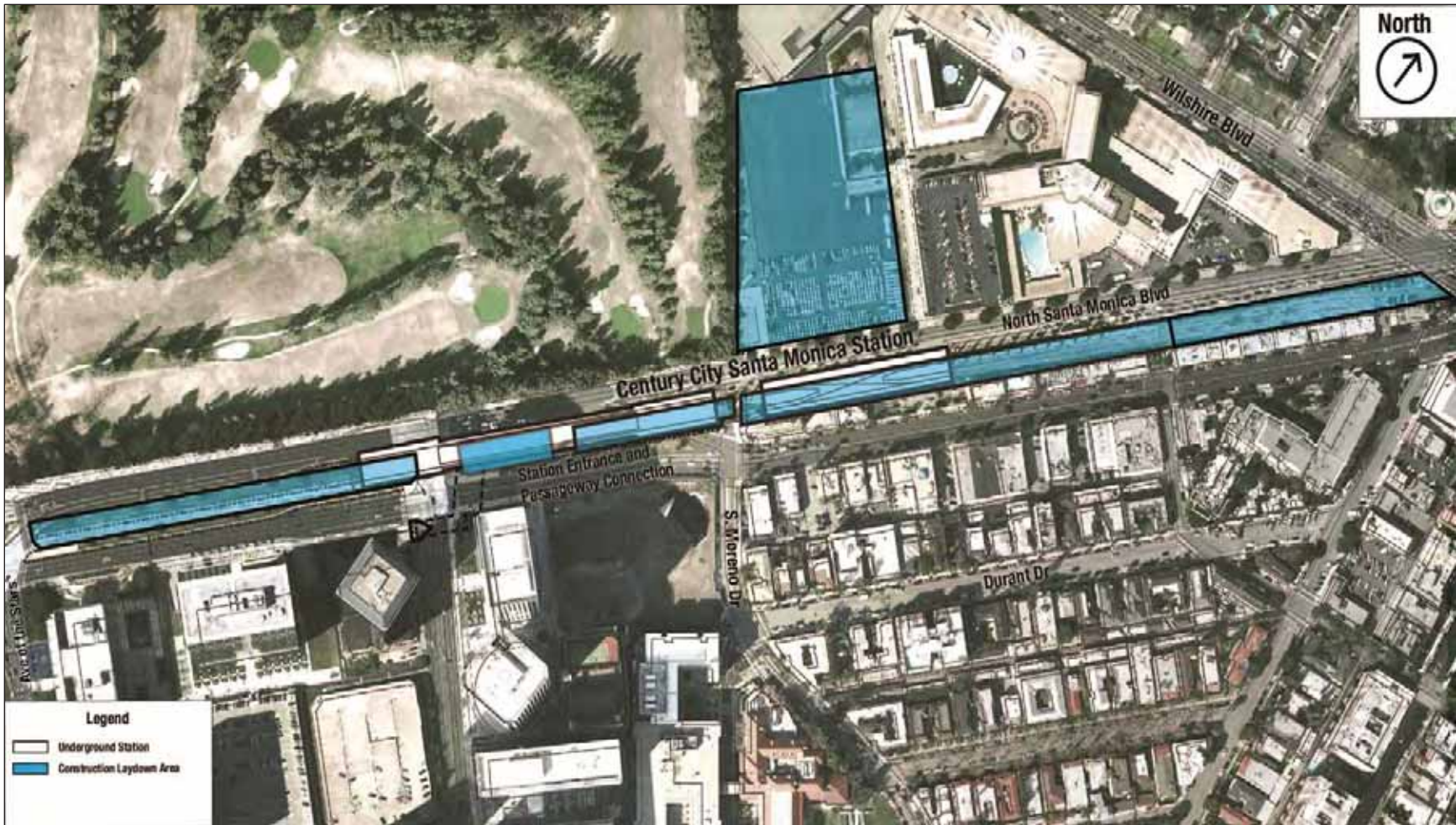
Century City Santa Monica Station – Construction Staging and Laydown Areas Scenario A
