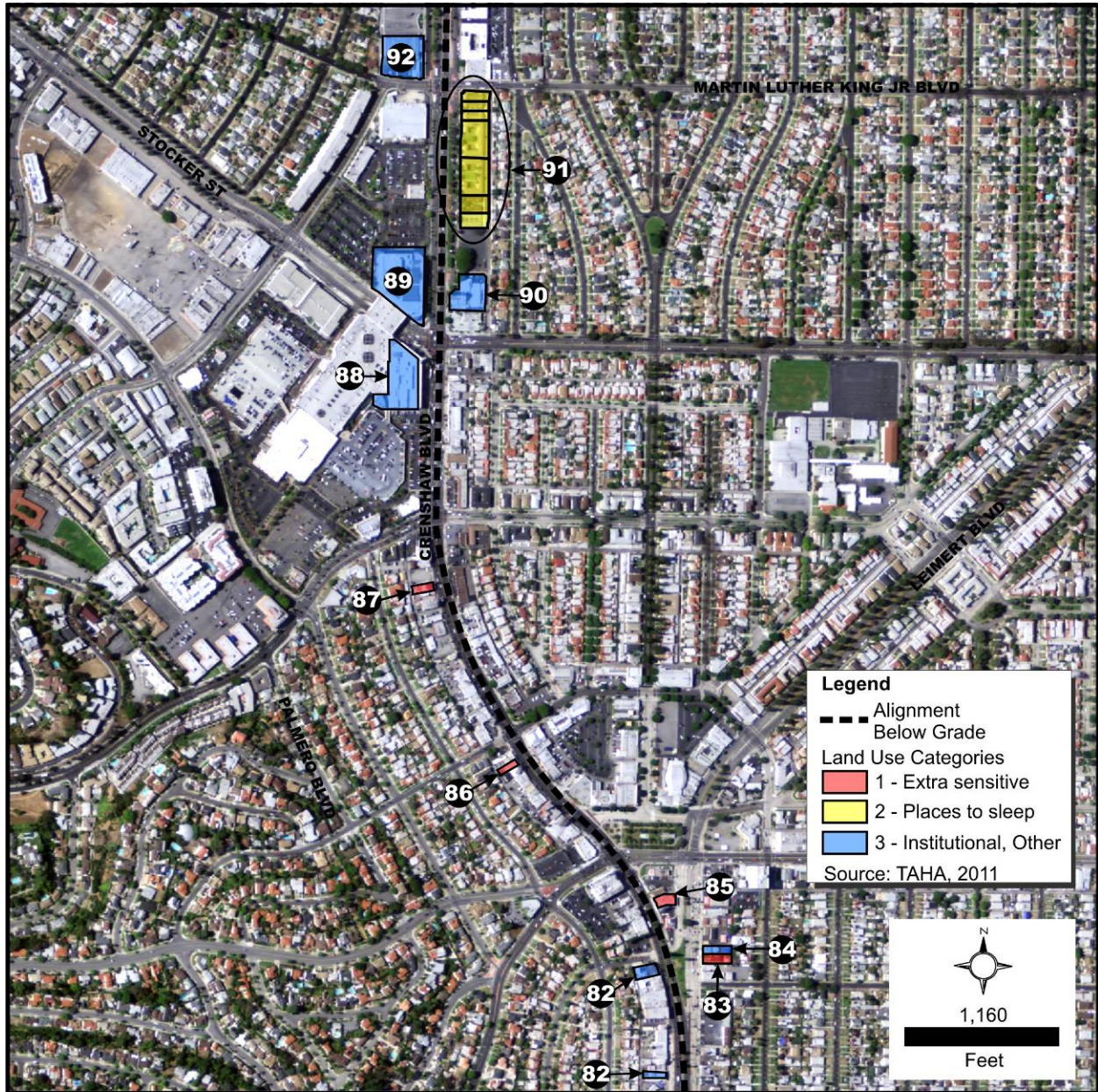
Figure 4-36. Noise-Sensitive Receptors – 48th Street to King Boulevard
