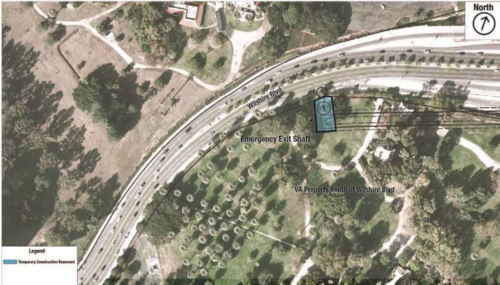
Figure 5-24: Westwood/VA Station South Vertical Shaft Easement
