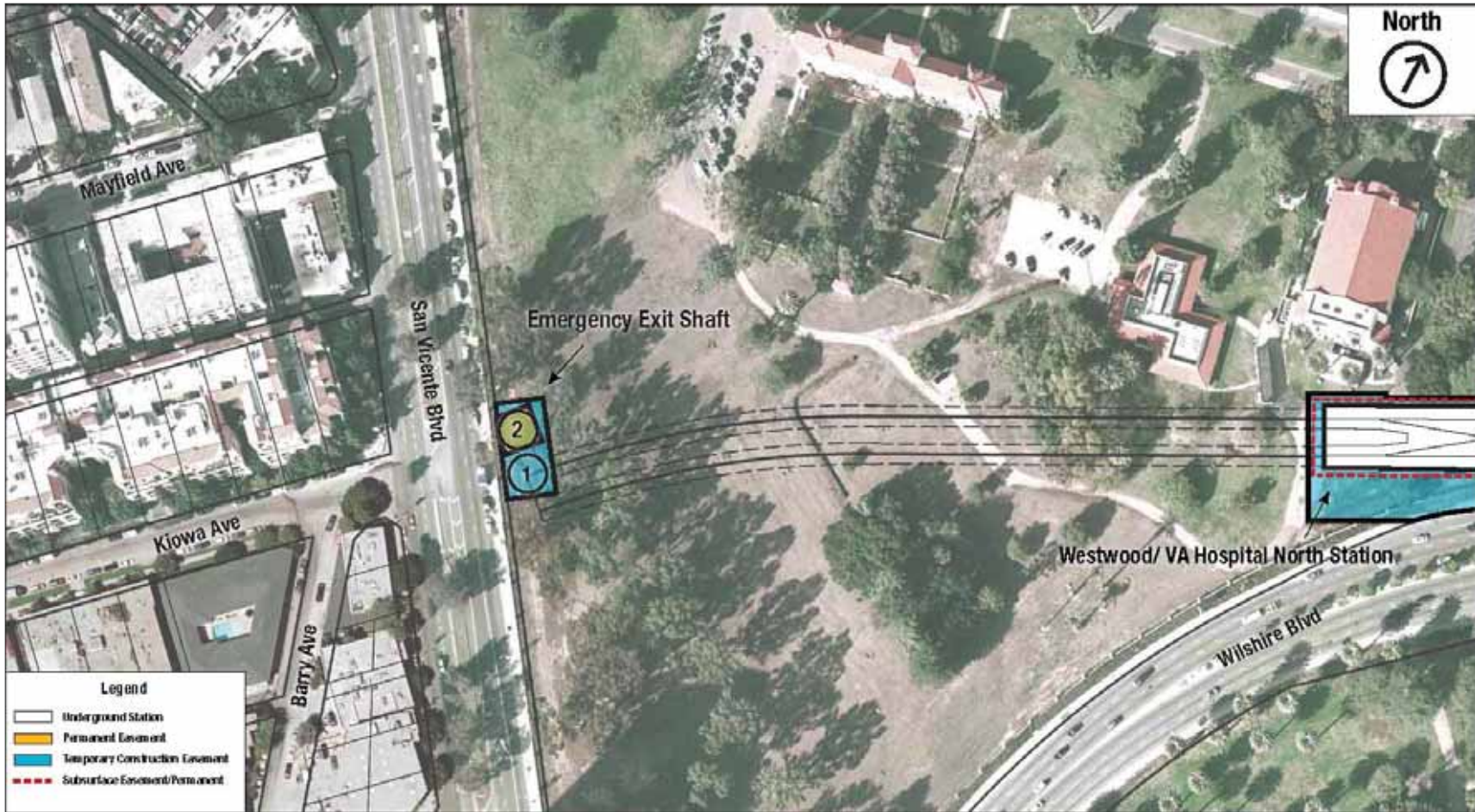
Figure 5-25: Westwood/VA Station North Vertical Shaft Easements
