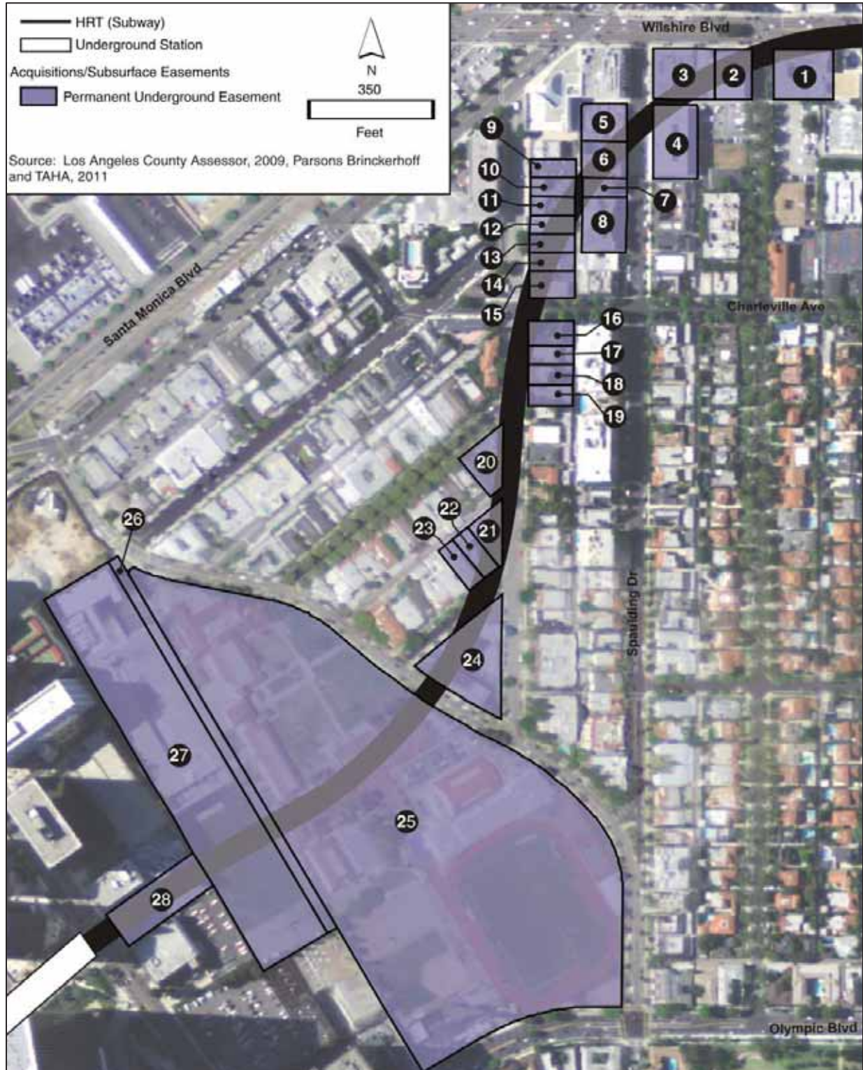
Figure 5-28: Permanent Underground Easements from the Wilshire/Rodeo Station to the Century City Constellation Station
