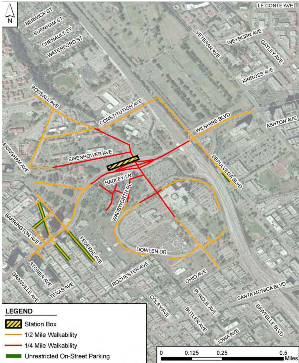
Figure 4-42 Unrestricted On-Street Parking— Westwood/VA Hospital Optional Station
