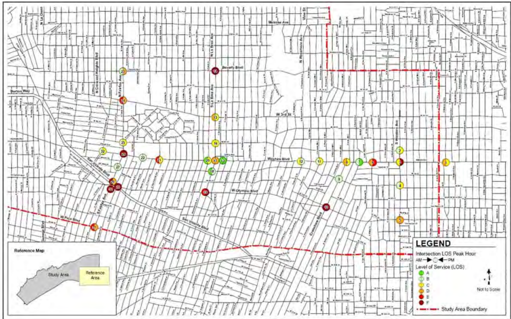
Figure 4-23. Existing Intersection Levels of Service
