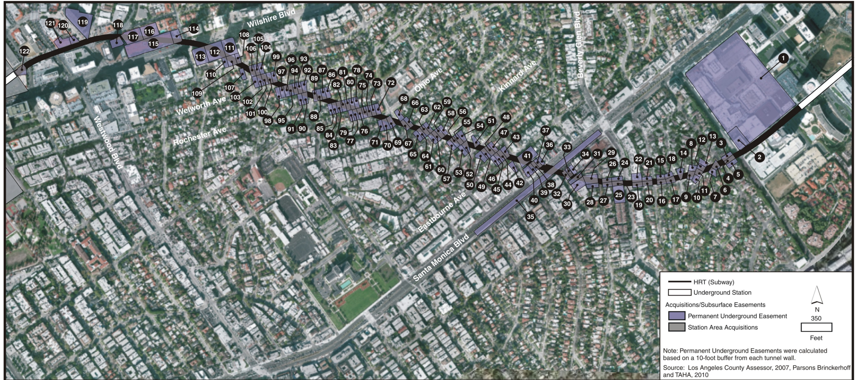
Figure 5-7: Segment Option 4R: Permanent Underground Easements
