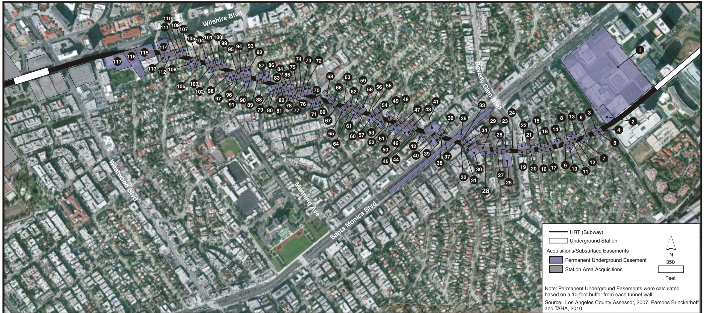
Figure 5-8: Segment Option 4S: Permanent Underground Easements
