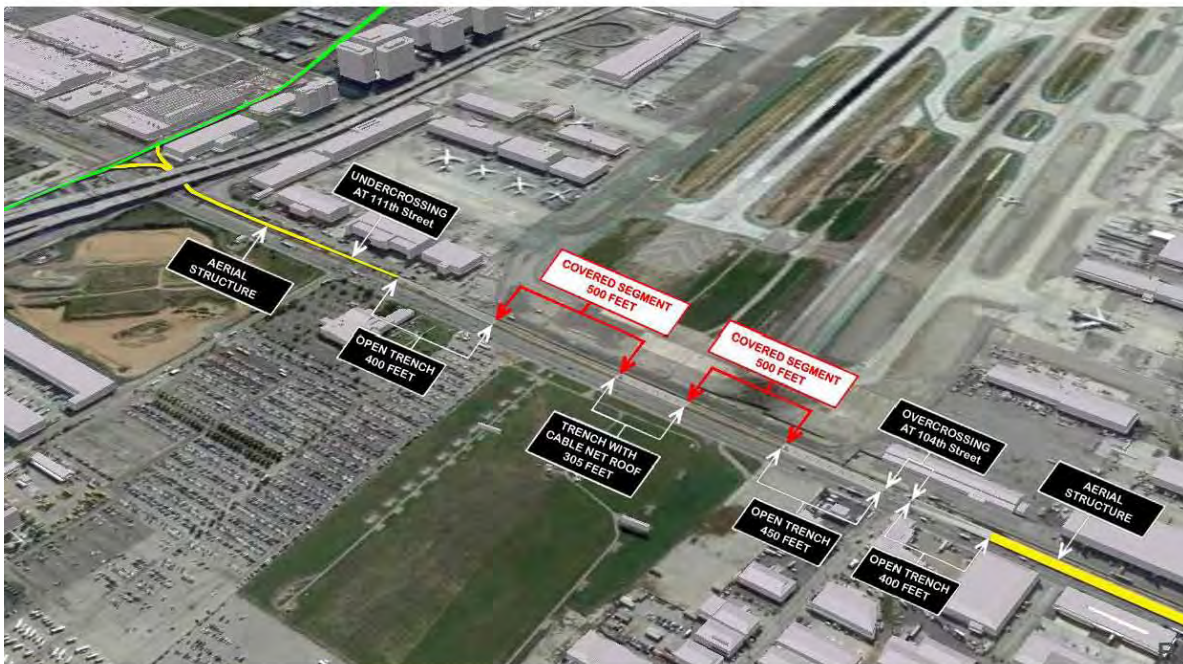
The Partially-Covered LAX Trench Option (interim solution) would be covered directly in front of the runways and have open sections in the middle and on the ends.
