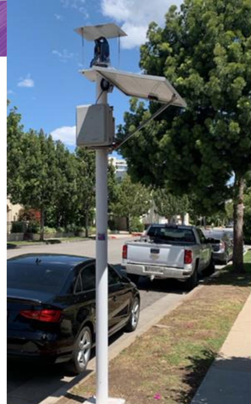
Example of 10-foot geotechnical instrumentation pole.
