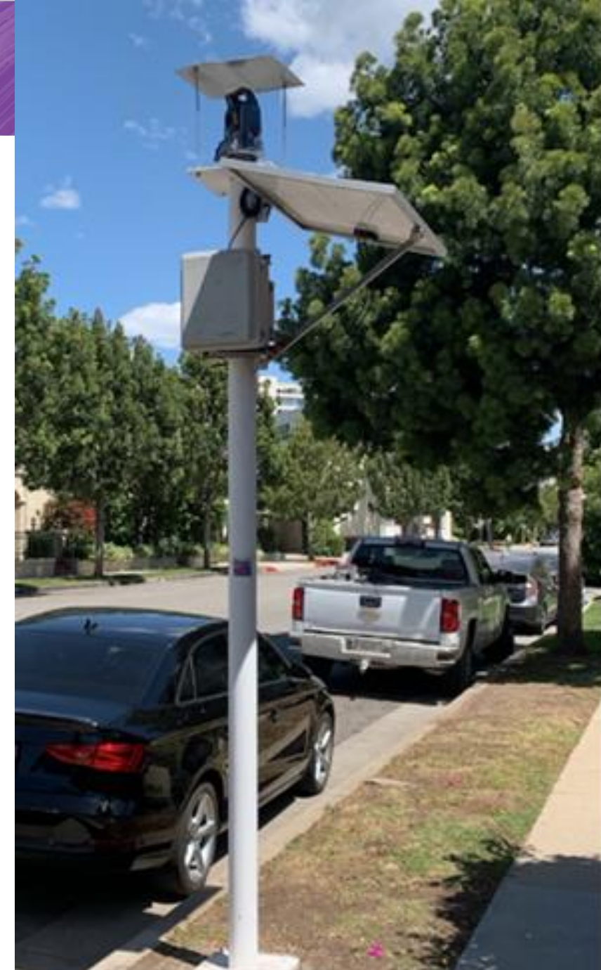
Example of 10-foot geotechnical instrumentation pole.
