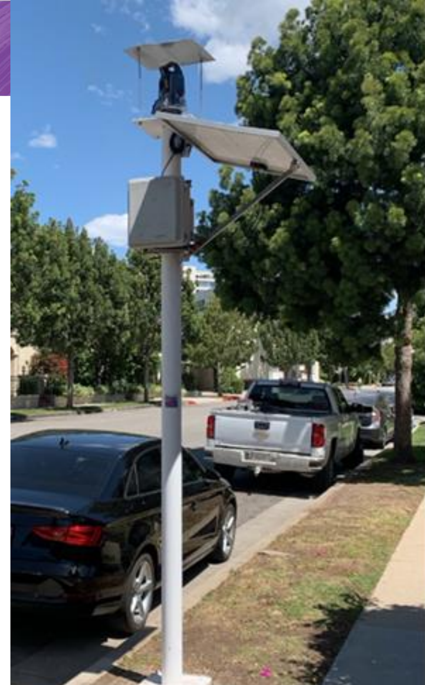
Example of 10-foot geotechnical instrumentation pole.
