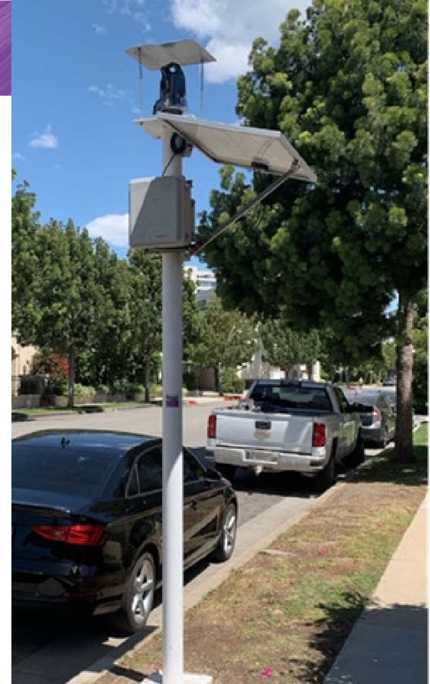
Example of 10-foot geotechnical instrumentation pole.
