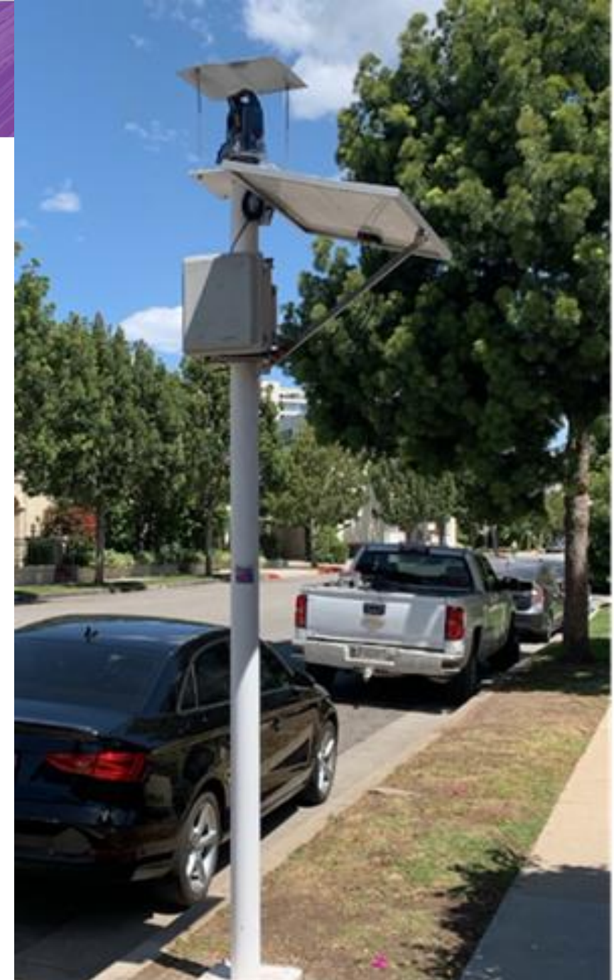
Example of 10-foot geotechnical instrumentation pole.
