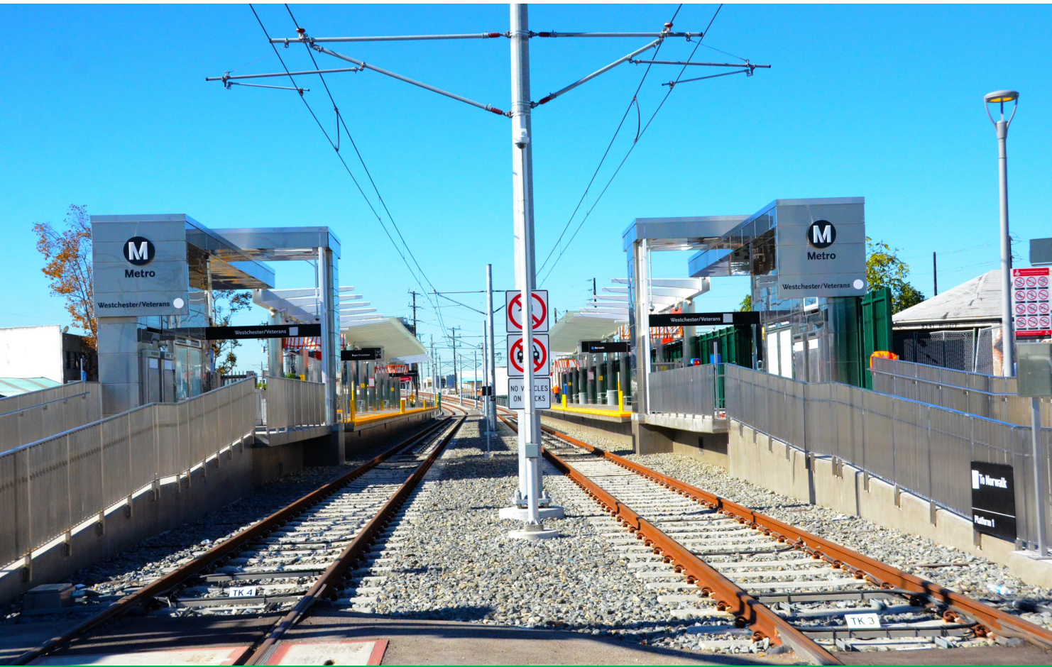
TVM canopy, Overhead Catenary System (OCS), railway track, and signage
