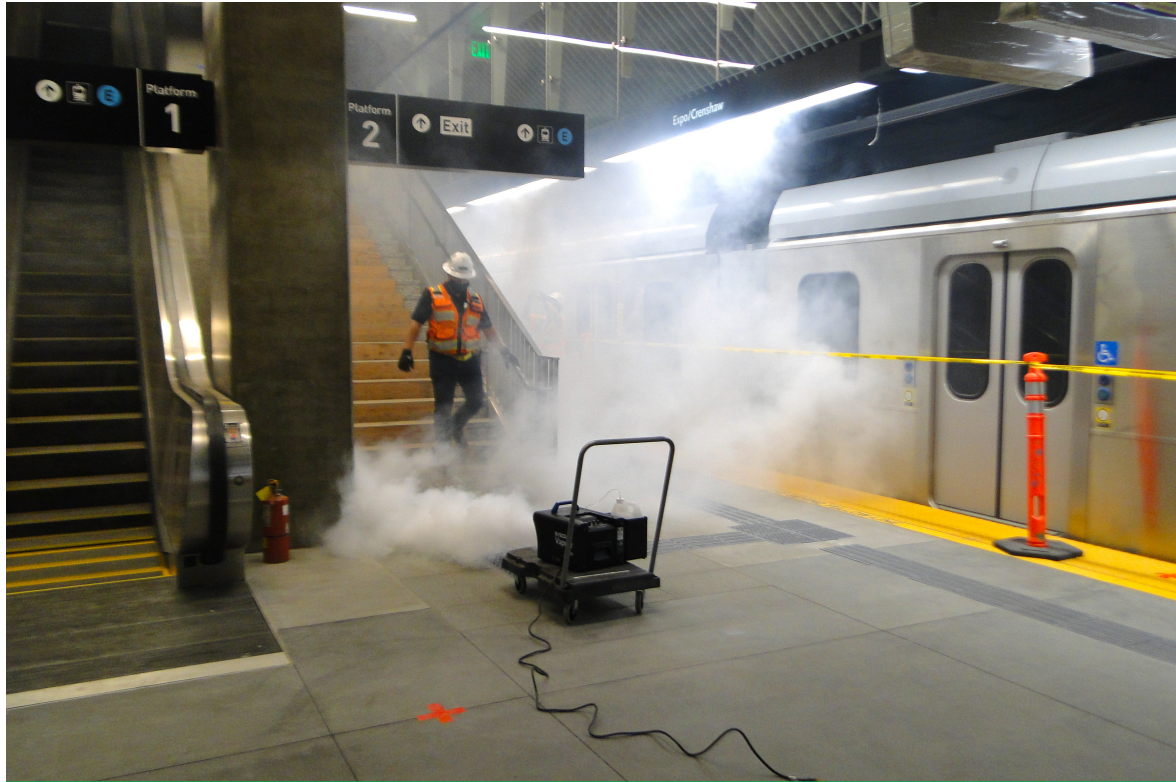
Smoke Test at Expo/Crenshaw Station
