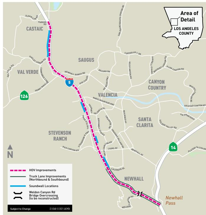
These enhancements will augment safety on the freeway by increasing access for merging and offering trucks a separate lane from the general-purpose lanes (GPLs) and are expected to provide a much faster and smoother driving experience in the area for locals and travelers. Additionally, they are part of a multi-phase program identified in Metro's Long Range Transportation Plan to ease congestion in LA County.
