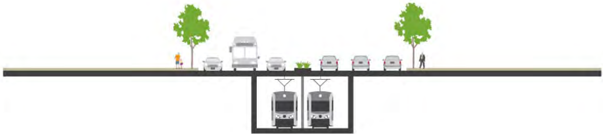
Figure 12: Below-Grade Cut-and-Cover Cross Section Example
