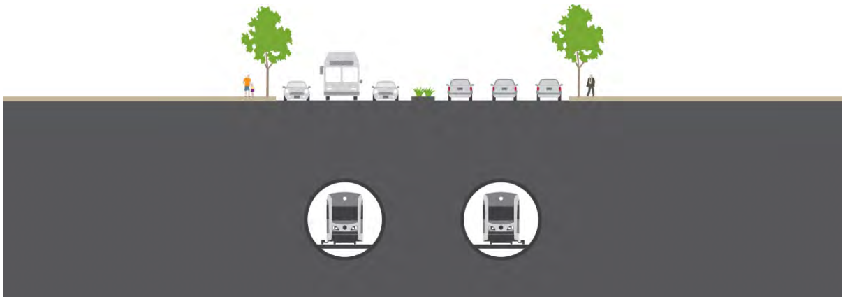
Figure 13: Below-Grade Bored Tunnels Cross Section Example
