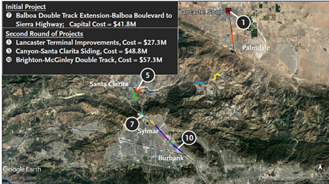
Figure 7-4: Recommended Capacity Infrastructure Projects
