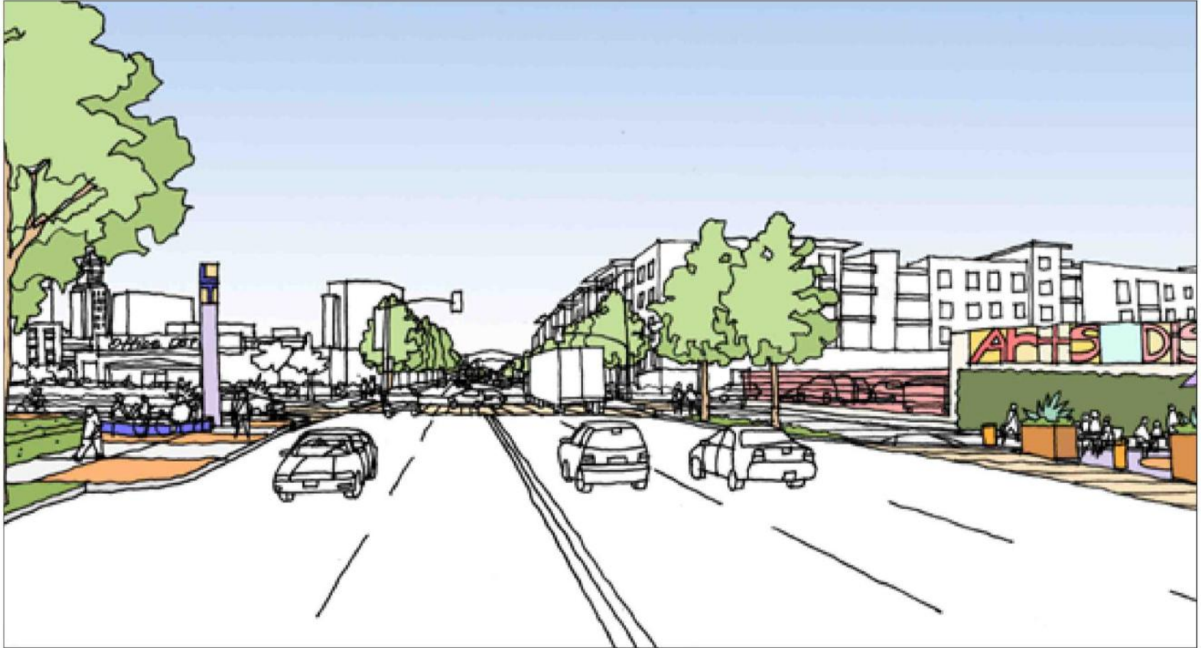
PROPOSED 2ND/TRACTION INTERSECTION Showing new plaza at 2nd St., People Street at Traction Ave., curb extensions to make a safer crossing of Alameda St.
