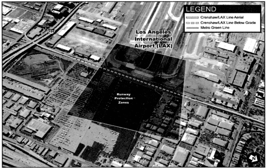
Below-grade trench alignment along Aviation Boulevard, adjacent to LAX south runways.
