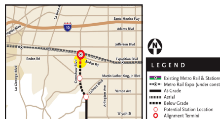
Design Option 6 is a below grade alignment along Crenshaw Boulevard between Exposition and 39th Street.
