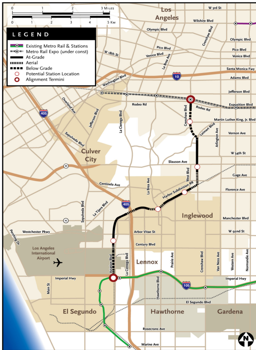
LPA Alignment. The LPA route is approximately 8.5 miles in length. It extends from the Exposition Light Rail line to the Green Line. This baseline option includes at grade, below grade and elevated sections, with six stations, as shown above.
