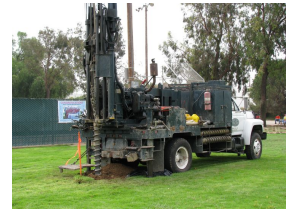
Continuous Core Drill Rig
