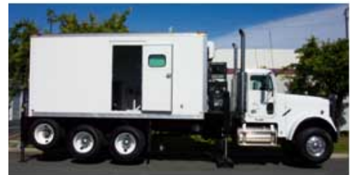
Cone Penetrometer Testing (CPT) Truck
