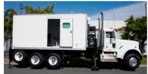
Cone Penetrometer Testing (CPT) Truck
